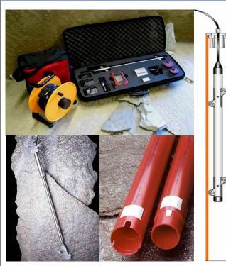
Systel Inclinometer Probe is used in conjunction with inclinometer casing for the measurement of lateral earth movements which might occur in unstable slopes, landslides, dam and roadway embankments, and landfills. They are also used to measure deflections in
